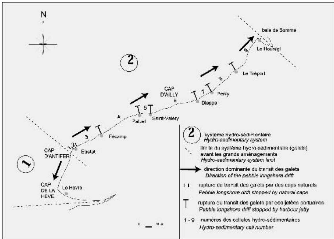
*Fig. 2 : Direction of the longshore transport and the hydro-sedimentary cells (Costa, 1997).*
