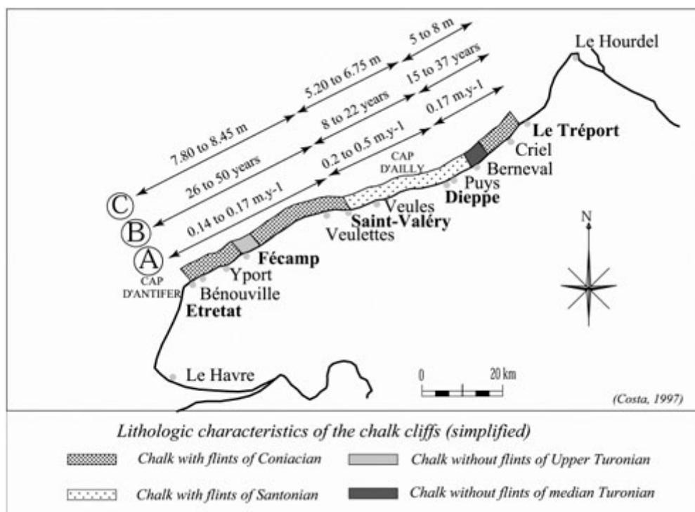
Fig. 8: Spatial location of the average chalk cliff retreat rate (A), the average repeat period of cliff falls (B), and the average per fall, in relation to the cliff toe stratigraphylithologic structure (C), per area between 1947 and 1995 (Costa, 1997).
