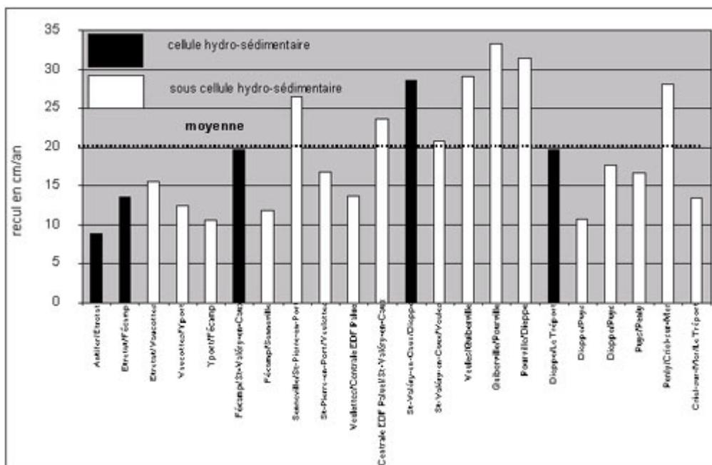
Fig.9: Haute-Normandie cliff erosion by hydrosedimentary cells between 1966 and 1995 (Costa, 2000 in CPIBP).
